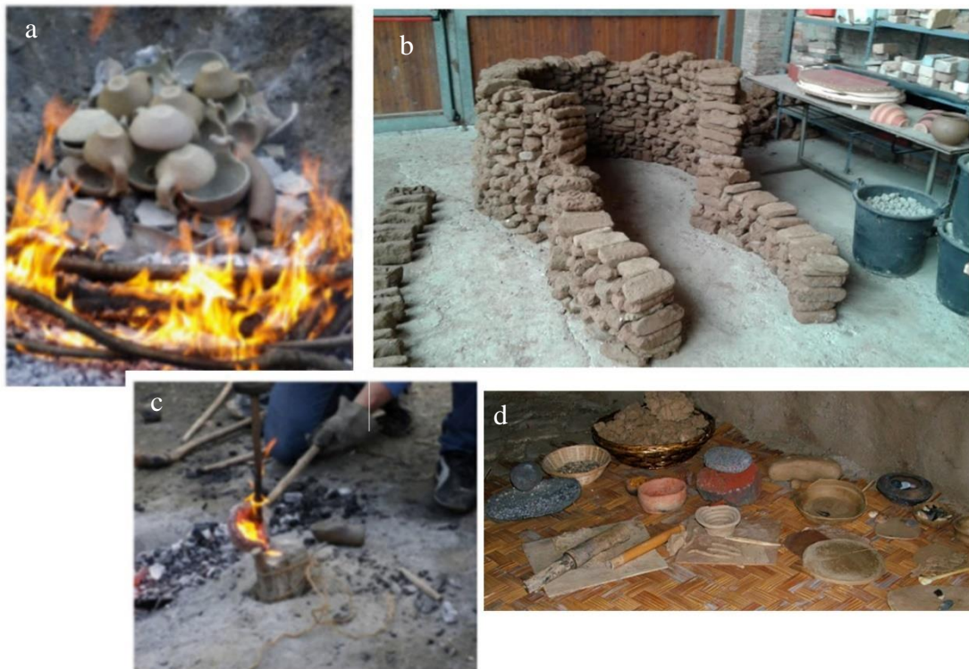
Figure 2: some images from the educational laboratories of several mentioned universities. a): experimenting with pottery cooking and bronze smelting (Cattani M., 2016); b): model of the kiln, currently being pre-recorded (LASERT, 2016); c): LAParS
