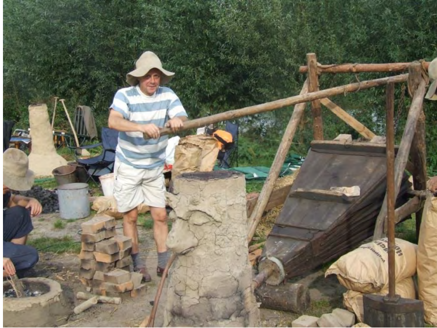
Figure 3: Experimenting with producing iron, Eindhoven Museum, the Netherlands
